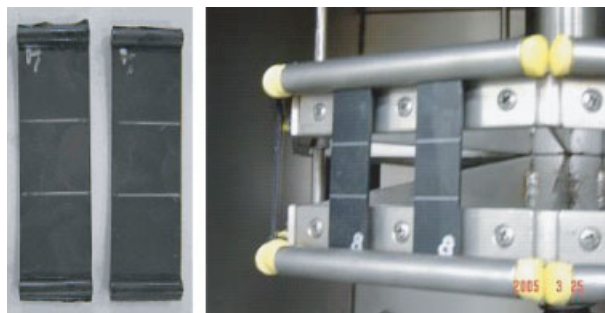
Figure 2 Test specimens and test configuration in dynamic ozone cabinet. [Color figure can be viewed in the online issue, which is available at www.interscience.wiley.com .]
